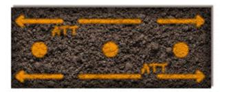
Duct structures marked in excess of 36 inches in total will require the underground facility notify the excavator and identify the size of the marked.
