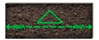
10. Single facilities, including direct buried facilities, should be marked by placing marks over the approximate center of the facility.
