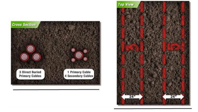
14. Multiple facilities of the same type other than electric that are bundled and intertwined in the same trench shall be marked over the approximate center of the facilities. The marks shall indicate the number of facilities in the corridor.
